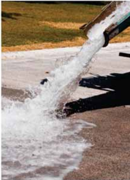
To illustrate the ability of the pavement to absorb water, Cemstone emptied a ready-mix truck full of water as fast as it could be dispatched. PHOTO: JOE NASVIK
